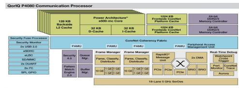
Core Complex (CPU, L2 and Frontside CoreNet Platform Cache)
